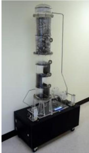
This working model is an impressive and dynamic educational piece of equipment! It dramatically demonstrates the operation of a column using water and air. The model's simulation is designed to show the basic process of distillation. Liquid traveling downward comes in contact with the vapors (gas bubbles) traveling upward, thus allowing the cooler liquid to condense any heavy compounds out of the lighter vapor stream.
