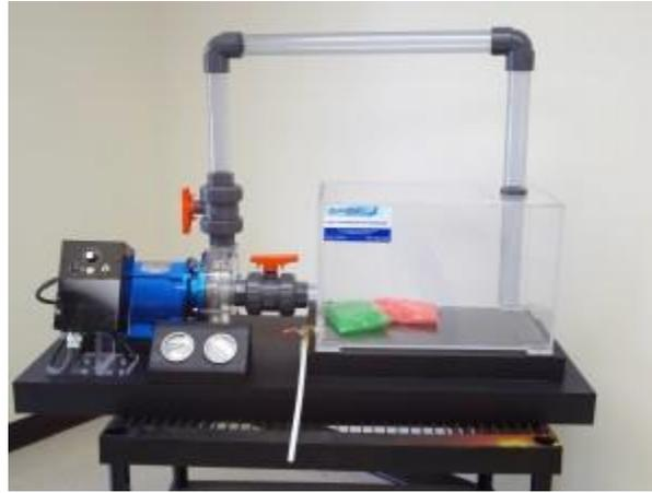
This “see through” training model has many features that can be used to train operators on the mechanical workings of a centrifugal pump. By manipulating the flow with suction and discharge valves and adjusting RPM's this model can demonstrate cavitation and other pump and flow phenomena. Our Pump Demonstration Model is a very popular tool for a site and sound concept of these workings, which cannot be experienced in the field or with drawings or computer simulations.
