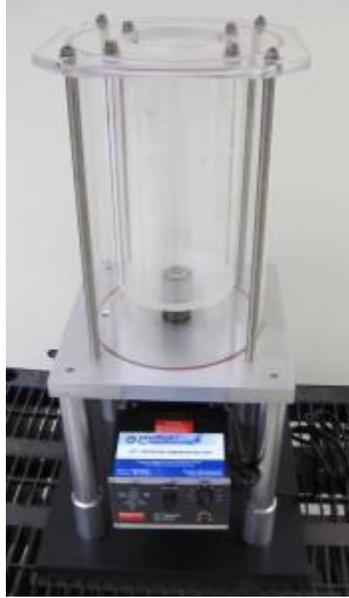
This acrylic model was designed and manufactured for the purpose of demonstrating separation of liquids from solids by means of centrifugal force. Both the inner and outer 'tubs' are see through acrylic and allow full visibility of the process.
