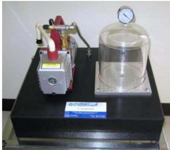
This acrylic model vividly demonstrates the effect of atmospheric pressure variations on fluids and gasses. A good example is the boiling temperature of water.
