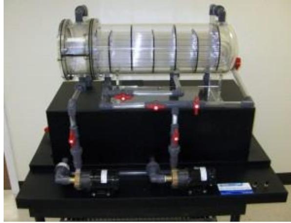
Table top working model has two (2) circulation pumps and two (2) supply tanks for demonstration. Different colored water streams will be circulated through the shell side and through the tube side to simulate the working of a real heat exchanger.
